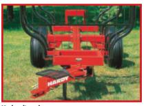
Hydraulic pole Models 3200DL and 5200DL have an articulated hydraulic pole to facilitate turning in tight spaces.
